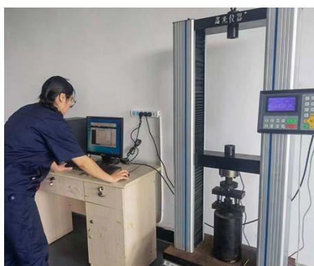
Bending Strength Inspection
