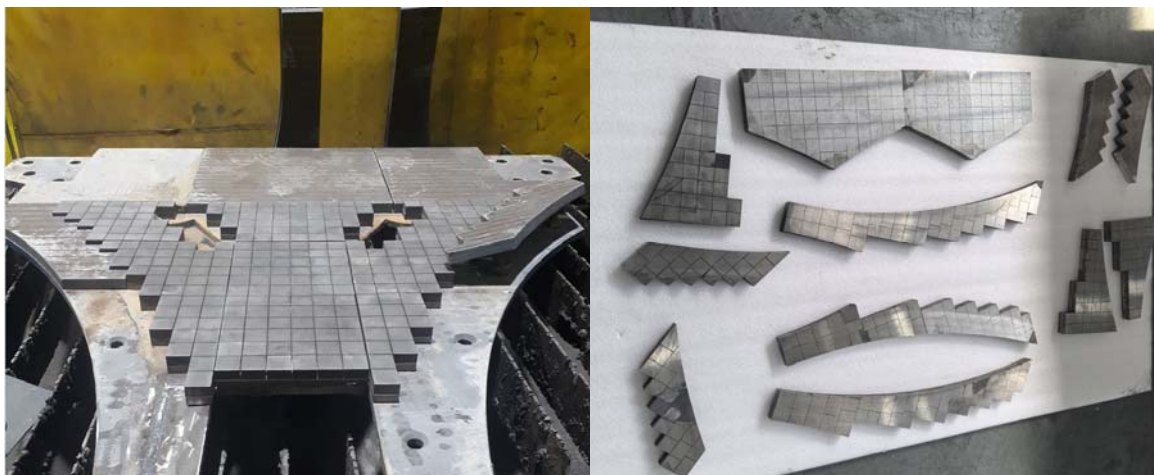
Liners for HPGR Feed Chute
