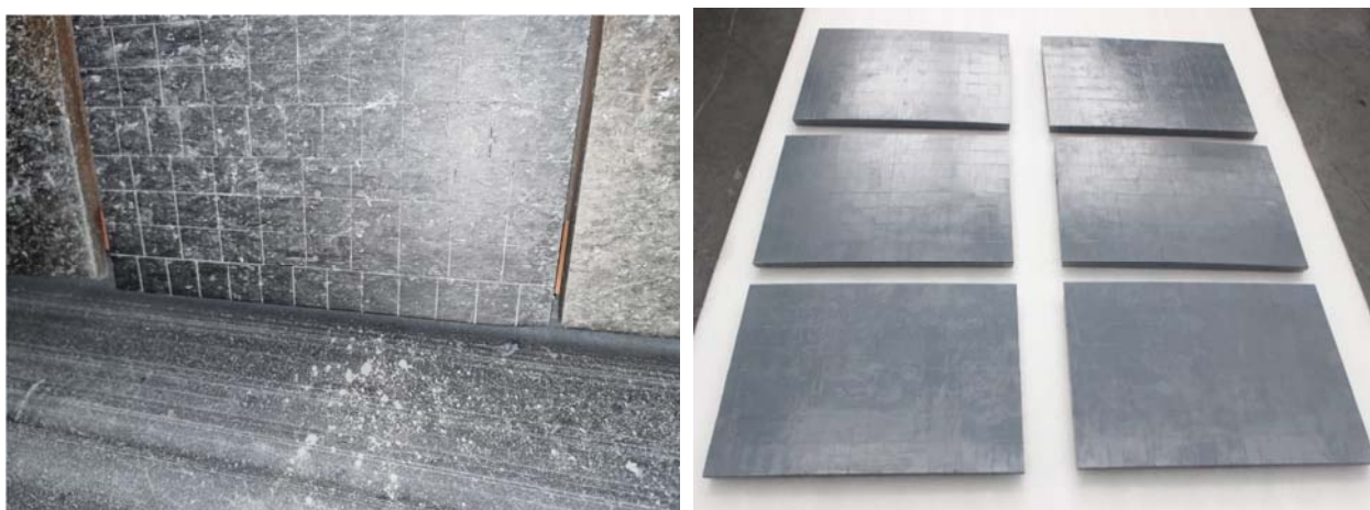
Drag liners for Transfer Conveyor
